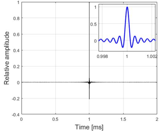
**Figure 2. Compressed Signal at Matched Filter Output**
