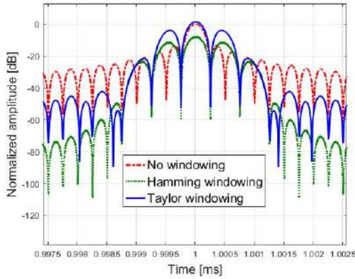
**Figure 3. Comparison between Two Well-Known Windowing Functions**
