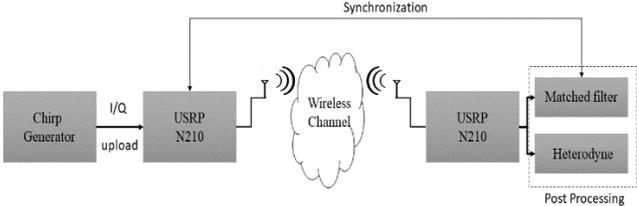
Figure 8. Block Diagram of SDR Sounding Experiment
