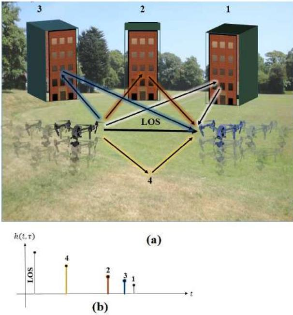
**Figure 5. Example Channel Environment with Example Impulse Response**
