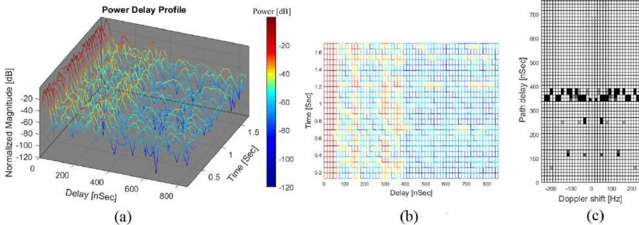
**Figure 6. Matched Filter Results: (a) PDP, (b) PDP Top View, and (c) Delay Doppler Spectrum**
